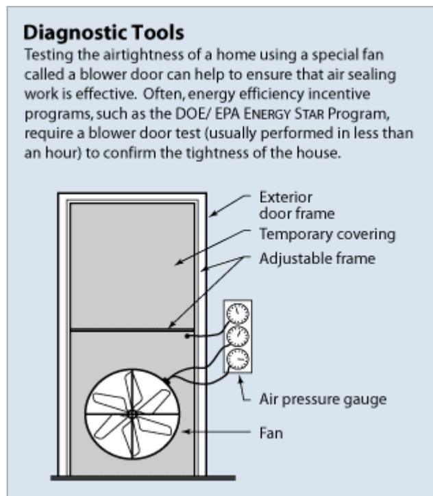
There are two types of blower doors: calibrated and uncalibrated. It is important that auditors use a calibrated door. This type of blower door has several gauges that measure the amount of air pulled out of the house by the fan. Uncalibrated blower doors can only locate leaks in homes. They provide no method for determining the overall tightness of a building. The calibrated blower door's data allow the auditor to quantify the amount of air leakage and the effectiveness of any air-sealing job.
